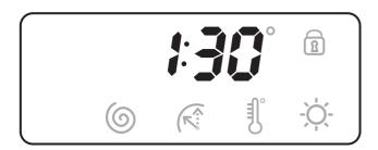
Once you have pressed the START/RESET button to start the programme, the display will indicate the amount of time left until the end of the wash cycle. If a delayed start has been set (using the Delay Timer, see page 9), the delay time will be indicated on the display.
